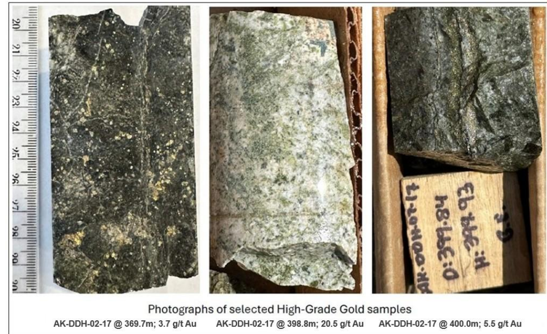
High-grade core samples taken from three different 3-meter sections from historical hole AK-DDH-02-17.
